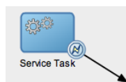
Figure A-44 The Error Catch Event as a Boundary Event on a Service Task
