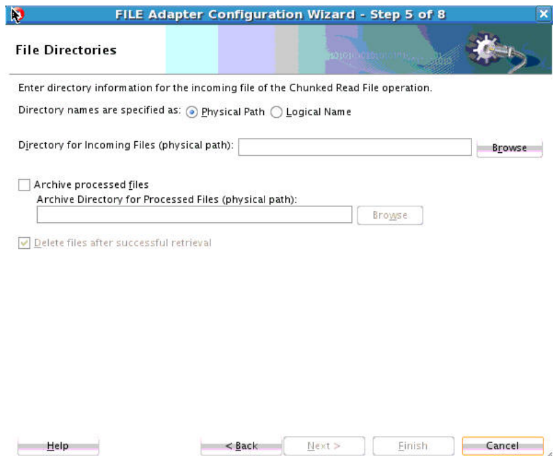
Figure 5-3 File Adapter Configuration Wizard Specifying the Directory Information for the Chunked Read Operation
