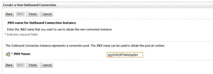
Figure 5-56 WebLogic Server Console Showing the JNDI Name for the New Instance Provided
