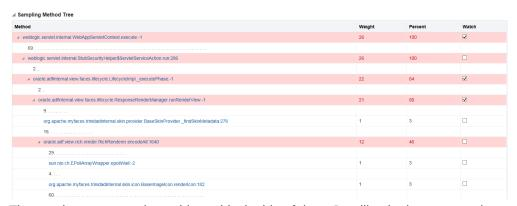
The tree is represented as a hierarchical table of data. Just like the instrumented tree, you can expand or collapse the methods inside the tree. Instead the table indicates the number of child processes. To see these methods, just click on the method. This opens the Method Calls Details dialog, which displays the complete call stack for this method. From this dialog you can select to watch any methods in the calling stack.
