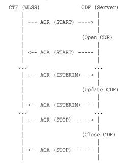
Here, ACA START is sent a receipt of a service request by Converged Application Server. ACA INTERIM is typically sent upon expiration of the AII timer. ACA STOP is issued upon request for service termination by Converged Application Server.
