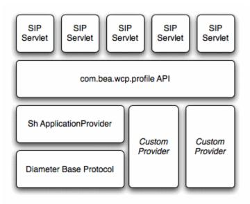
Figure 2–1 Profile Service API and Sh Provider Implementation
