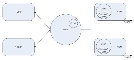
The SLRM supports any number of cores. In the diagram below, the SLRM services both Core1 and Core2. There are 2 Oracle Communications Core Session Managers for each core. The SLRM load balances registrations from P-CSCFs for Core1 between the Oracle Communications Core Session Managers at the top of the diagram and those for Core2 between the bottom.
