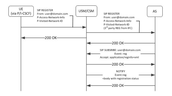
This feature is relevant when the Oracle Communications Core Session Manager is performing S-CSCF functions. You enable this feature on the Oracle Communications Core Session Manager per registrar, by simply creating a profile and applying it to the applicable registrar.
