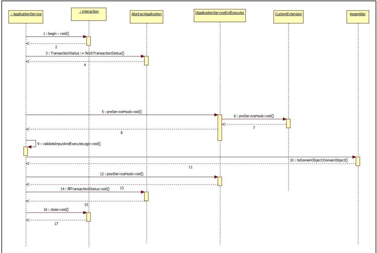
The pre hook is provided after the invocation of *fetchTransactionStatus* call inside the application service. At this step, the current task code is received, any additional manipulation of the input received from the User interface channel can be done in the pre hook. Apart from this additional data coming from the screen specific to client requirements can be handled in the pre hook.
