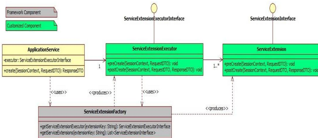
**Note:** The RequestDTO and ResponseDTO components depicted in above diagram are explained in subsequent sections. For now, note that the RequestDTO contains inputs to the application service method and ResponseDTO contains output generated by the method.
