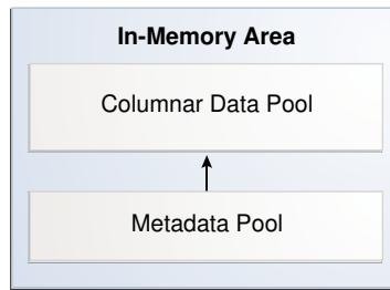
The database determines the relative size of the two subpools using internal heuristics. The database allocates the majority of space in the In-Memory Area to the columnar data pool (1 MB pool).
