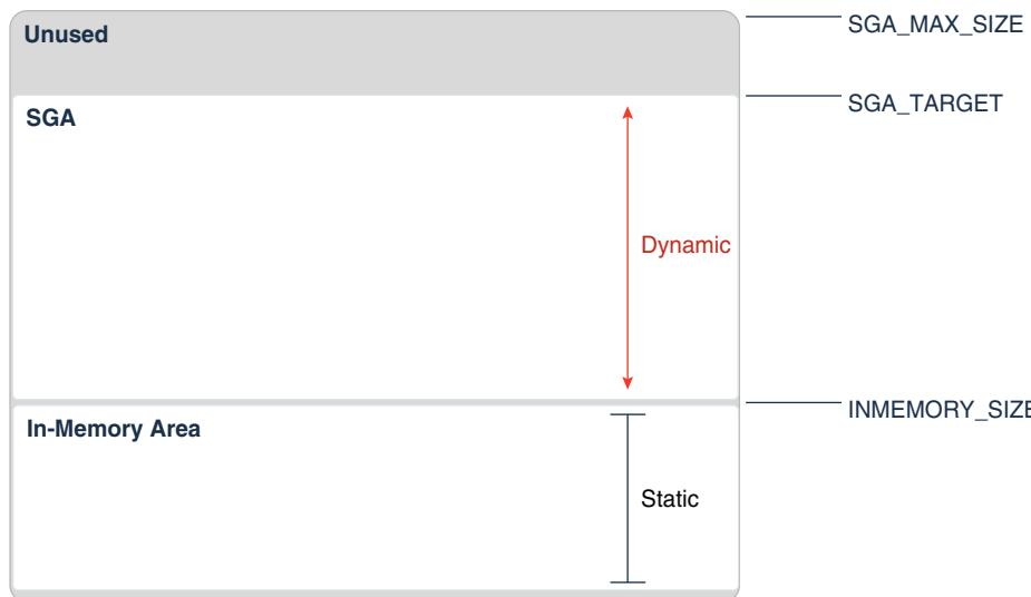
Unlike the other components of the SGA, including the buffer cache and the shared pool, the In-Memory Area size is not controlled by automatic memory management. The database does not automatically shrink the In-Memory Area when the buffer cache or shared pool requires more memory, or increase the In-Memory Area when it runs out of space.
