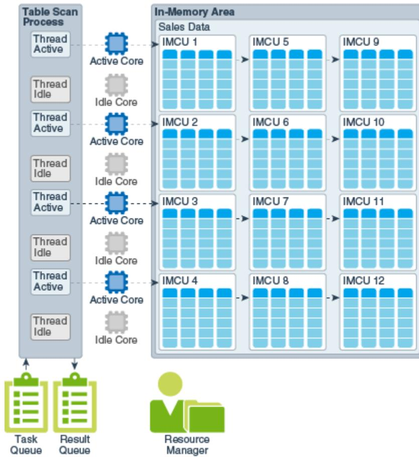
In the preceding graphic, the database host has 8 CPU cores. Based on an internal algorithm, Resource Manager assigns 4 threads to assist the table scan process. In this scenario, 4 CPU cores remain idle for other concurrent database operations to use.
