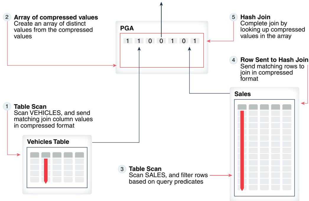
As illustrated in the preceding diagram, the database performs a hash join on the compressed data as follows:
