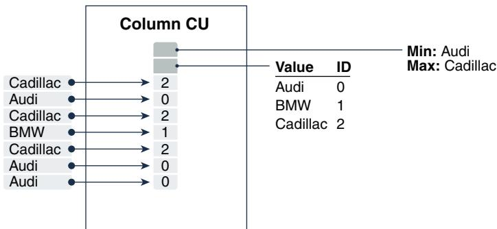
In the preceding figure, the CU contains only 7 rows. Every distinct value in this CU, such as Cadillac or Audi, is assigned a different dictionary code, such as 2 for Cadillac and 0 for Audi. The CU stores the dictionary code rather than the original value.
