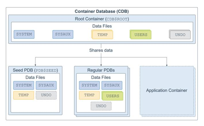
A database is a set of physical files that store user data and metadata. The metadata consists of structural, configuration, and control information about the database server. You can design your database to be a multitenant container database (CDB) or a non-container database (non-CDB).
