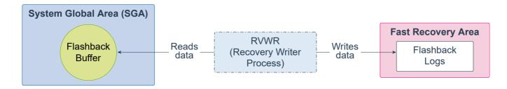
Recovery Writer Process (RVWR) is a background process that is used to flashback an entire database. That is, it undoes transactions from the current state of the database to a time in the past, provided you have the required flashback logs. When flashback is enabled or when there are guaranteed restore points, RVWR writes flashback data to flashback database logs in the fast recovery area.
