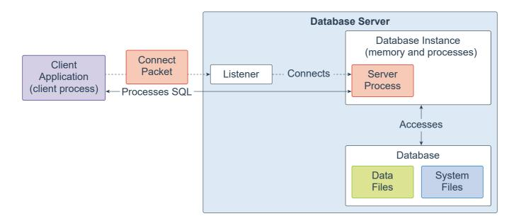
An Oracle Database consists of at least one database instance and one database. The database instance handles memory and processes. The database consists of physical files called data files, and can be a non-container database or a multitenant container database. An Oracle Database also uses several database system files during its operation.
