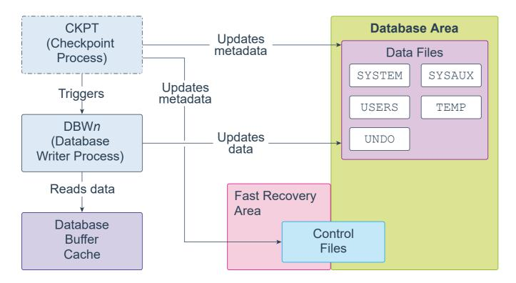
Checkpoint Process (CKPT) is a background process that, at specific times, starts a checkpoint request by messaging Database Writer Process (DBWn) to begin writing dirty buffers. On completion of individual checkpoint requests, CKPT updates data file headers and control files to record the most recent checkpoint.
