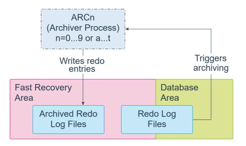
Archiver Processes (ARCn) are background processes that exist only when the database is in ARCHIVELOG mode and automatic archiving is enabled, in which case ARCn automatically archives online redo log files. Log Writer Process (LGWR) cannot reuse and overwrite an online redo log group until it has been archived.
