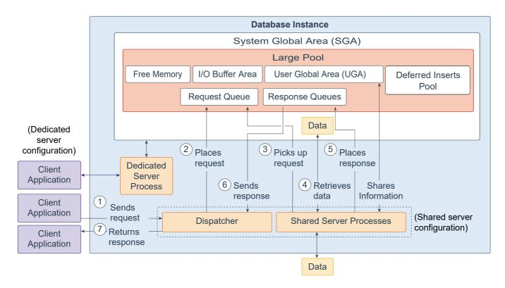
The large pool is an optional memory area that database administrator's can configure to provide large memory allocations for the following:
