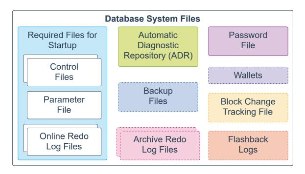
The following database system files are used during the operation of an Oracle Database and reside on the database server. Note that data files are physical files that belong to database containers and are not described here.
