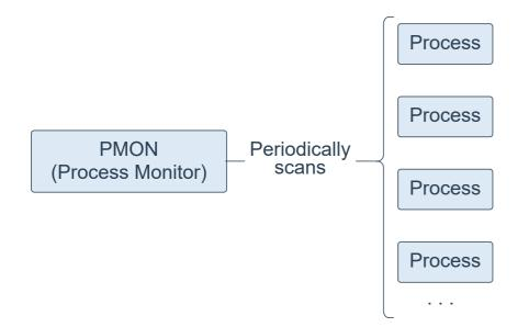
Process Monitor Process (PMON) is a background process that periodically scans all processes to find any that have died abnormally. PMON is then responsible for coordinating cleanup performed by the Cleanup Main Process (CLMN) and the Cleanup Slave Process slaves (CLnn).
