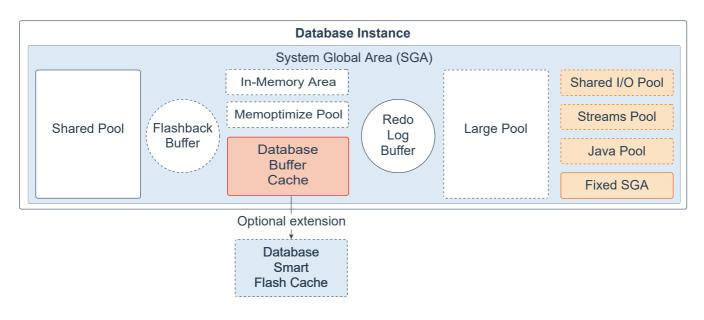
The System Global Area (SGA) is the memory area that contains data and control information for one Oracle Database instance. All server and background processes share the SGA. When you start a database instance, the amount of memory allocated for the SGA is displayed. The SGA includes the following data structures:
