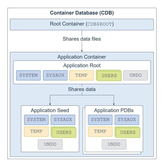
An application container is an optional, user-created CDB component that stores data and metadata for application PDBs. A CDB can include zero or more application containers. An application container consists of exactly one application root and one or more application PDBs, which plug into the CDB root. An application root belongs to the CDB root and no other container, and stores the common metadata and data.
