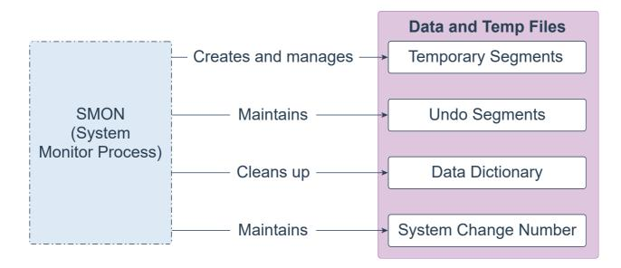
System Monitor Process (SMON) is a background process that performs many database maintenance tasks, including the following:
