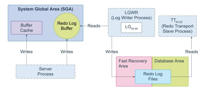
Log Writer Process (LGWR) is a background process that writes redo log entries sequentially into a redo log file. Redo log entries are generated in the redo log buffer of the System Global Area (SGA). If the database has a multiplexed redo log, then LGWR writes the same redo log entries to all of the members of a redo log file group.
