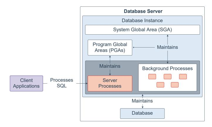
A database instance contains a set of Oracle Database background processes and memory structures. The main memory structures are the System Global Area (SGA) and the Program Global Areas (PGAs). The background processes operate on the stored data (data files) in the database and use the memory structures to do their work. A database instance exists only in memory.
