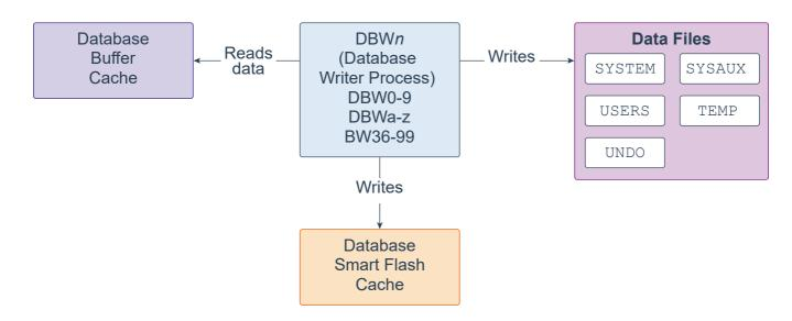
Database Writer Process (DBWn) is a background process that primarily writes data blocks to disk. It also handles checkpoints, file open synchronization, and logging of Block Written records. DBWn also writes to the Database Smart Flash Cache (Flash Cache), when Flash Cache is configured.
