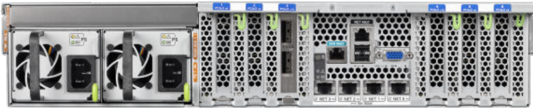
Figure A-39 Rear View of Extreme Flash Exadata Storage Server X5-2 Servers
