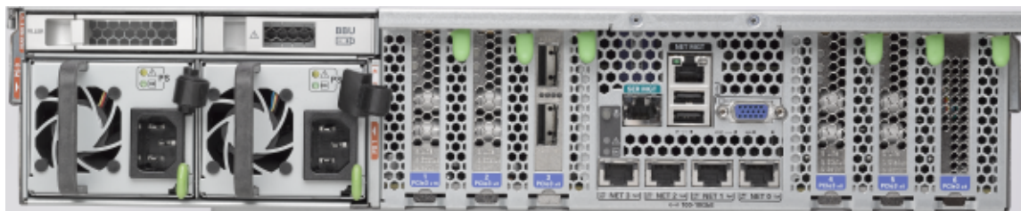
Figure A-41 Rear View of Exadata Storage Server X4-2L Servers
