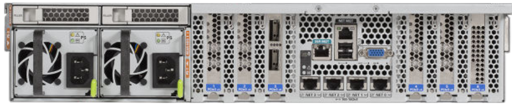
Figure A-43 Rear View of Exadata Storage Server X3-2L Servers
