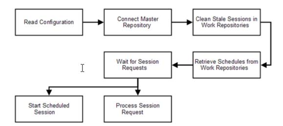
Figure 4-1 Oracle Data Integrator Agent Startup Cycle
