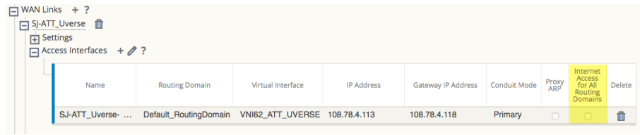
Figure 8: Enabling Internet access for All Routing Domains
