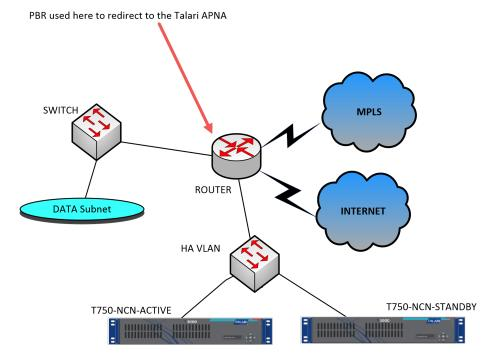
VLAN or subnet as the Active appliance and the router, as we show in the diagram below:
