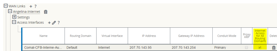
Figure 8: Enabling Internet access for All Routing Domains
