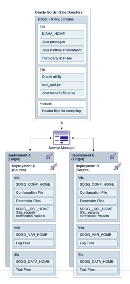
The following table describes the key MA directories and the variables that are used when referring to those directories in an Oracle GoldenGate installation. When you see these variables in an example or procedure, replace the variable with the full path to the corresponding directory path in your enterprise topology.
