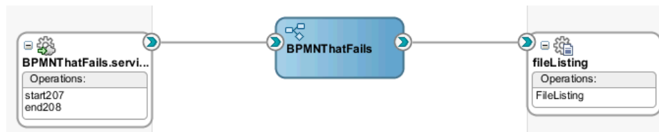
Figure 19-2 Composite with BPMN Process Service Component
