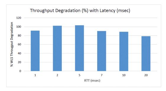
Figure 6-1 Throughput Degradation With Latency in a Stretch Cluster
