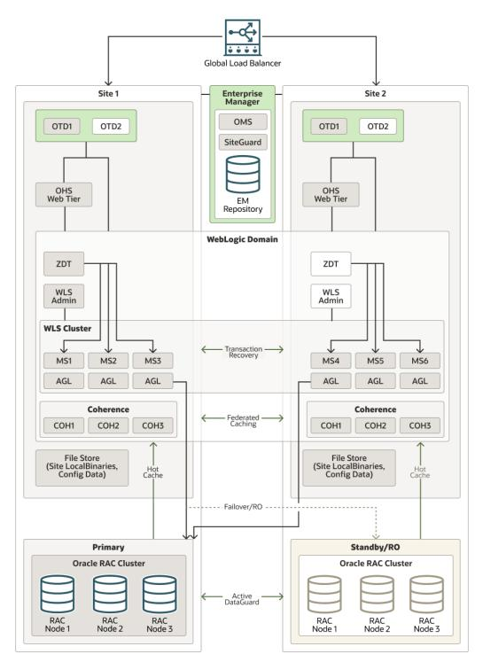
Figure 2-3 Topology for an Active-Active Stretch Cluster Application Infrastructure Tier and an Active-Passive Database Tier
