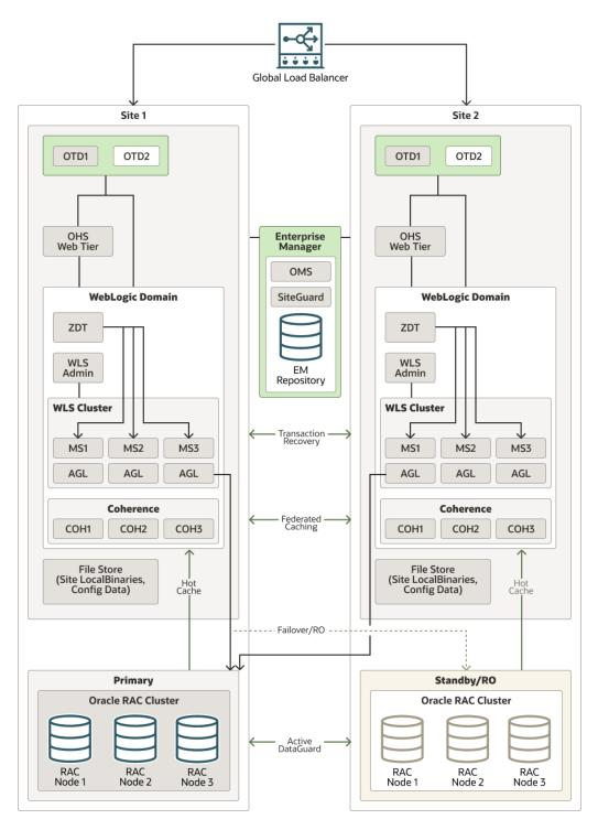
Figure 2-1 Topology for an Active-Active Application Infrastructure Tier with an Active-Passive Database Tier
