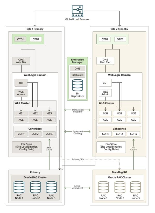
Figure 2-2 Topology for an Active-Passive Application infrastructure Tier with an Active-Passive Database Tier
