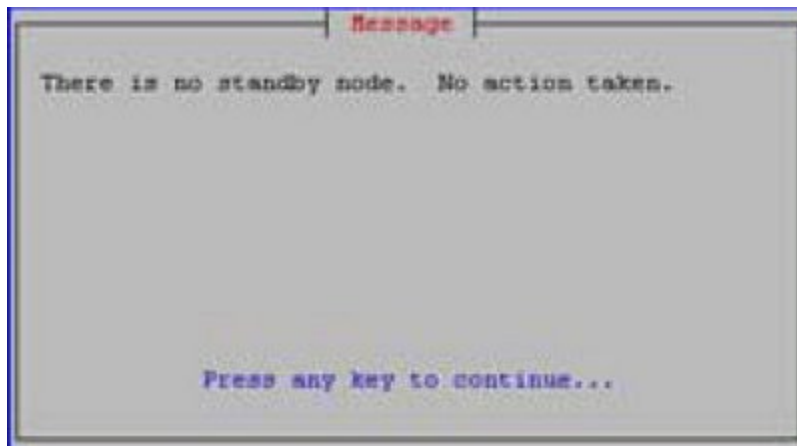
Figure 6-1 Unable to Switchover to Standby
