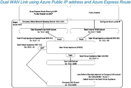
Figure 2. Sample Topology for Single WAN Link using Azure Express Route
