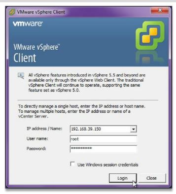
Figure 2: Enter IP address, User name, and Password
