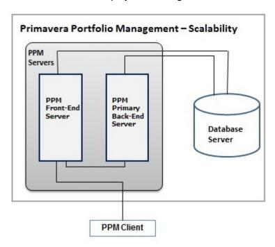
For Small deployments, include a secondary back-end server. This is suggested as a result of testing with the data set described in *Appendix A*.
