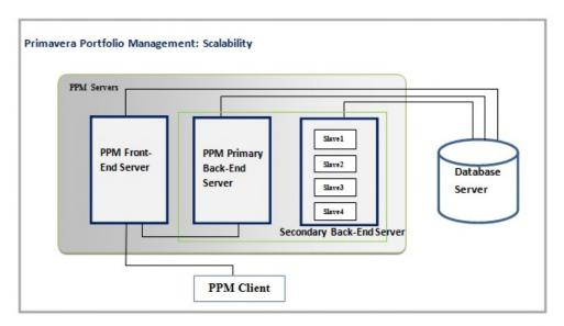
You can manage increasing complexity by adding additional servers (secondary back-end and front-end servers). For database servers, the number of nodes in RAC implementation must be increased, as shown in the figure below:
