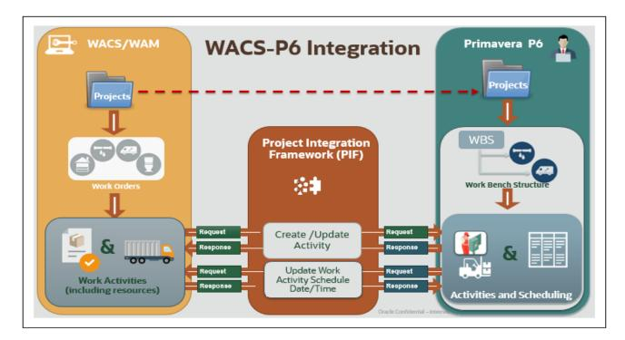
In this integration, Project Integration Framework is used as a middleware to connect the applications. It uses REST APIs to facilitate communication between these two applications.
