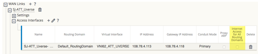
Figure 8: Enabling Internet access for All Routing Domains
