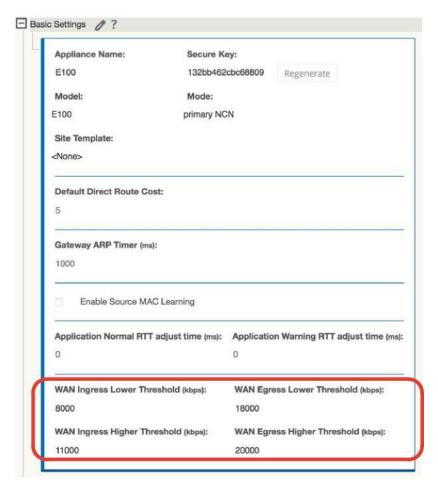
When a threshold is configured and the combined WAN link usage for the site exceeds the configured value, an event will be generated.
