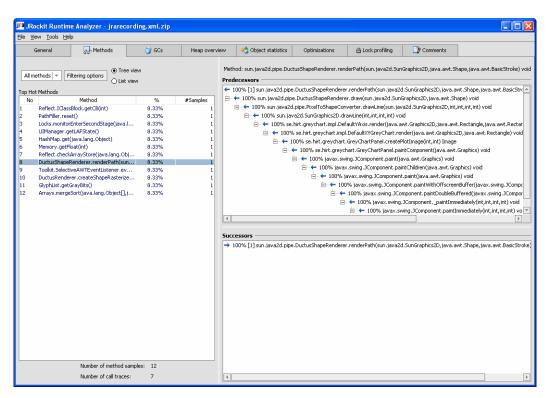
The hot methods data is collected periodically by JRockit sampling the running threads and looking at which method the threads are executing. If your recording has native sampling enabled, you can also see methods prefixed by jvm#, which are native methods in the JVM. You can limit the methods shown in the top list by clicking **Filtering options** and select the least number of samples that you want displayed.
