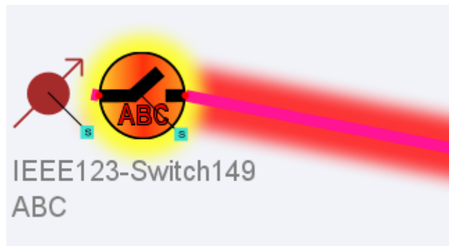
Example: Switch Warning and Conductor Violation
