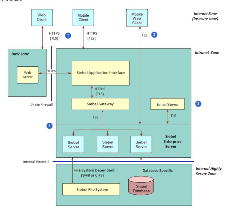
The encryption mechanisms illustrated in this image are as follows:
