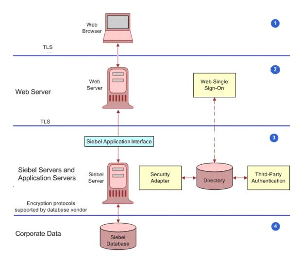
This figure shows that communications encryption is available between the following:
