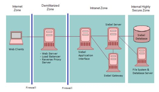
As illustrated in this figure, an enterprise network for Siebel CRM typically comprises the following zones of control:
