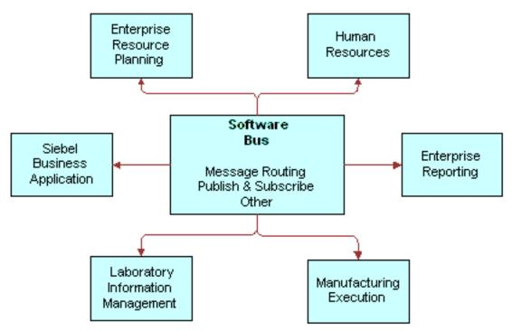
An enterprise can adopt a software bus strategy for application integration. Master data is partitioned across systems, and the software bus middleware implements a messaging architecture to exchange application data. The messaging functionality ranges from simple message routing, in batch or real time, to a publish and subscribe scheme.
