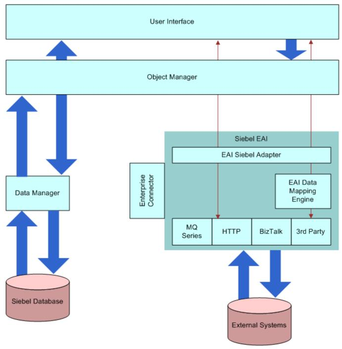
Because data management functions are abstracted to the object layer, declarative configuration can be used instead of a procedural configuration, such as scripting. Declarative configuration improves and simplifies configuration work while lowering the costs associated with maintenance.
