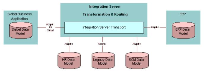
A Siebel application can integrate with an integration server by using an adapter provided by a partner, such as IBM, TIBCO, or WebMethods. For information about supported integration servers, see Siebel System Requirements and Supported Platforms.
