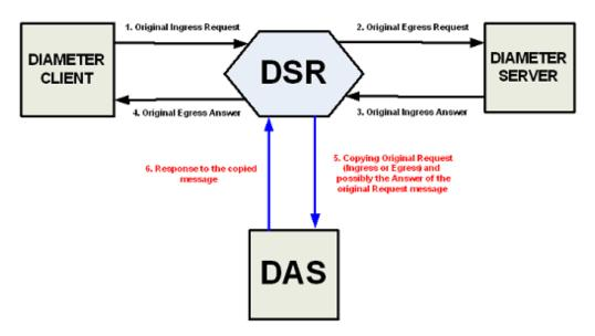
Figure 11-1 Diameter Message Copy Message Flow
