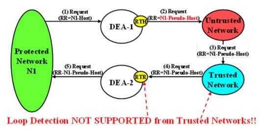
Figure 9-9 Unsupported Pseudo-Host Route-Record Loop Detection
