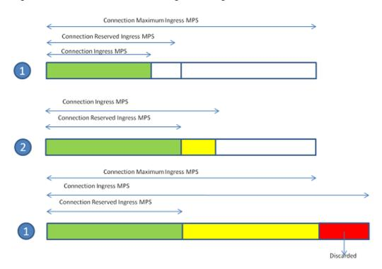
Figure 12-1 Per-Connection Message Coloring
