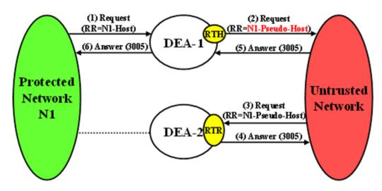
Figure 9-8 Multi-DEA Route-Record Message Loop Detection
