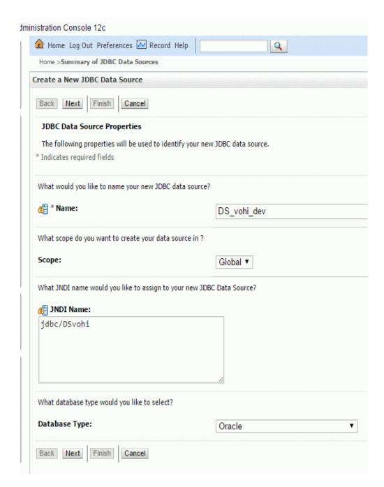
Next you need to specify a database driver. For regular database instances, use "Oracle's Driver (Thin) for Service connections; Versions: Any".
