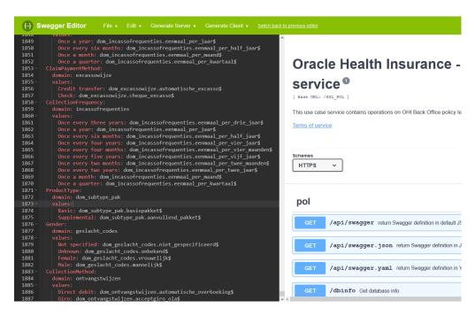
You can now navigate through the paths, operations and type definitions of the HSL service. More information about Swagger can be found on <a href="http://swagger.io">http://swagger.io</a>
