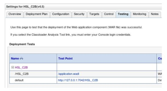
Also note that, even with the correct URLs, you cannot use a browser to test, because the request needs to send a Request Header "Accept:application/json".
