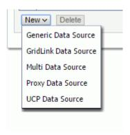
When the data source connects to a RAC data source it is more useful to choose for 'GridLink Data Source' as this can respond to instance state changes.
