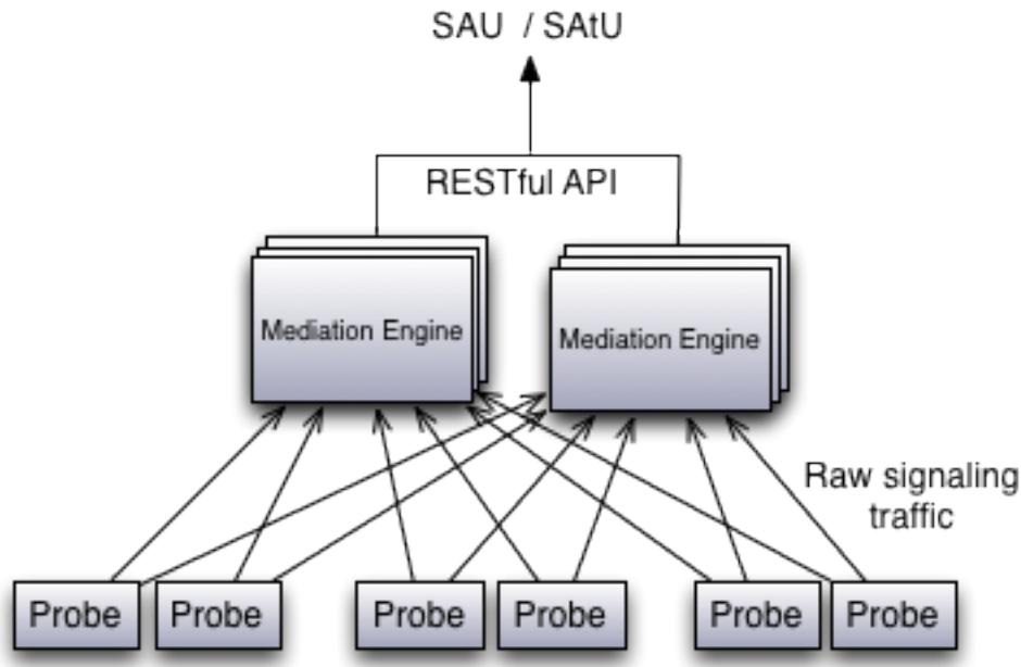
In this case, the RESTful API for exporting the KPIs is served directly by the ME machines (no aggregation step is needed). The same RESTful API is used by both the AE and the ME, so the application that interrogates it doesn't need to know if the Session Monitor setup is using an AE or not.
