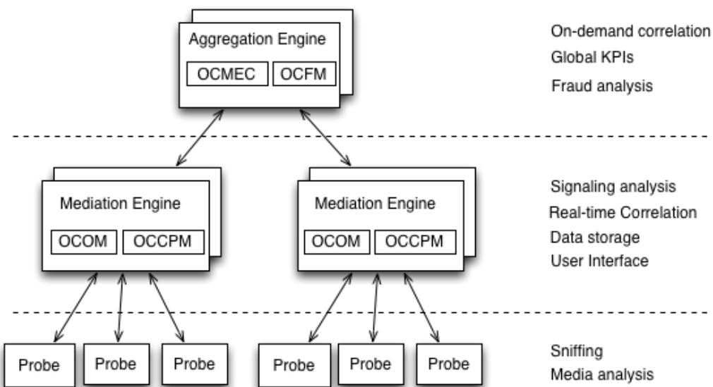
Each of the three layers supports high-availability by deploying two identical servers in active-passive or active-active modes of operation. For small setups, it is possible to run the probe
