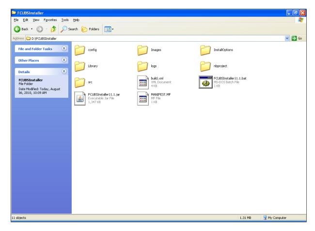
Inside the folder 'logs', you will find the log file 'FCUBSInstaller.log'. This file contains detailed information about the methods executed.
