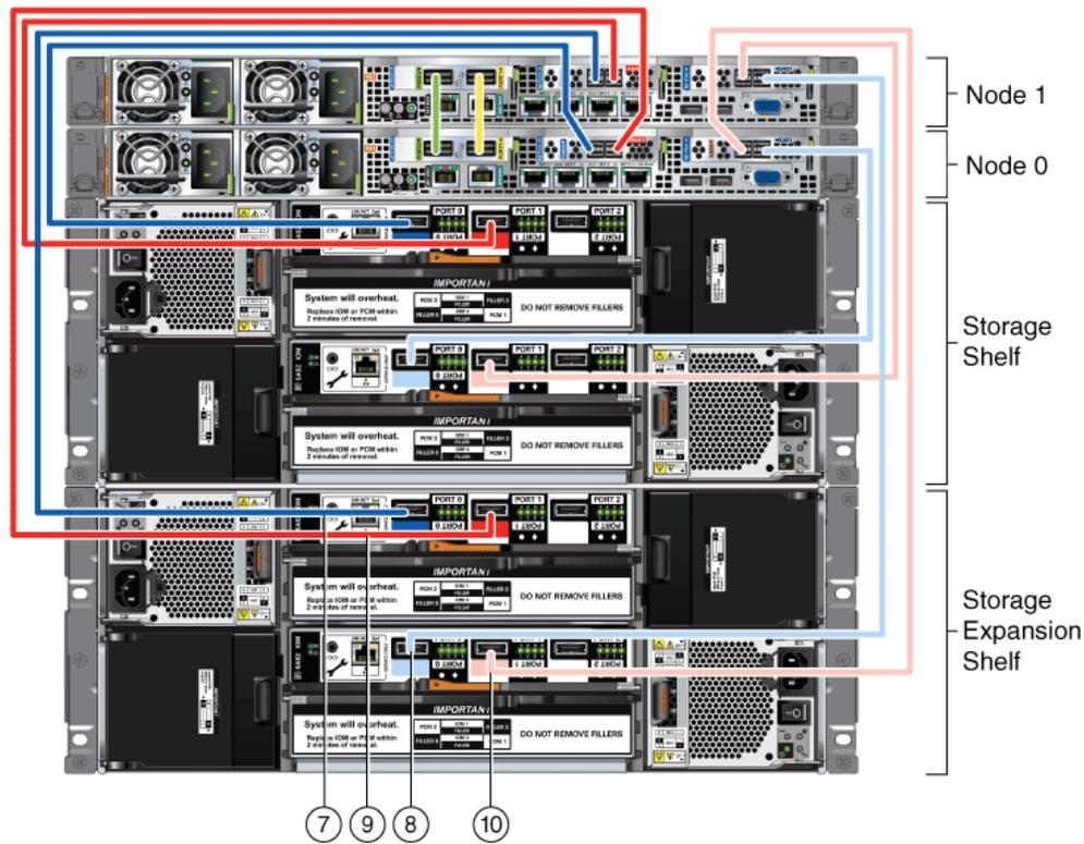
The cables identified with callout numbers in the preceding figures are included with each shipped Oracle Database Appliance storage expansion shelf. These cables are all black, but have colored labels at each end that match the references to cable colors in the text and the label colors on the back panels.
