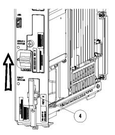
Figure 4-1 E5-APP-B Card Inject Hardware Switch, UNLOCKED
