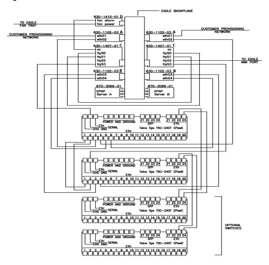
Figure A-1 EPAP Network Connections
