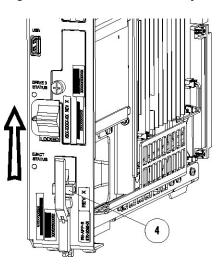
Figure 4-5 E5-APP-B Card Eject Hardware Switch, UNLOCKED
