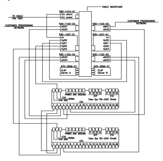
Figure A-4 ELAP Network Connections
