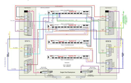
Figure A-2 Sync Network Redundancy (Eth04 used for Sync Network) Interconnectivity
