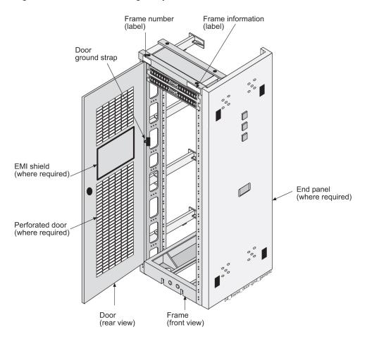
Figure 2-4 Door Grounding Strap Placement
