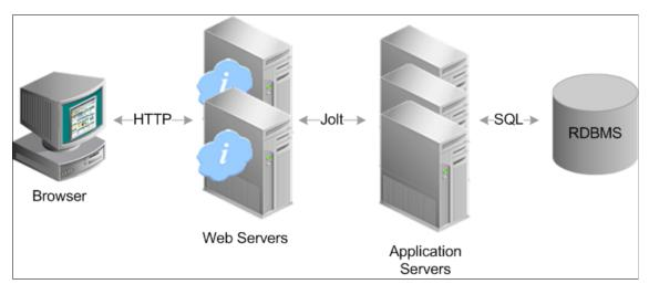
Within a PeopleSoft system, you can configure multiple PeopleSoft Internet Architecture installations on a web server as well as configure multiple domains on a single application server machine. If you reach the resource limits of a single server machine, you can incorporate more server machines to house
