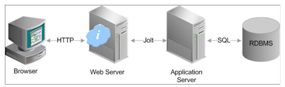
If the application server and database server don't reside on the same machine, then the application server and the database server should be connected to the same high-performance, backbone network. This ensures optimum performance.
