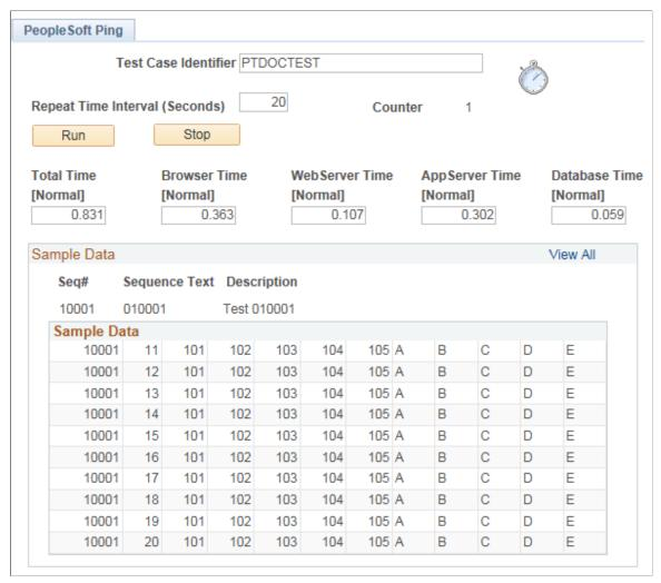
Enter a Test Case Identifier to uniquely group each set of metrics. For Repeat Time Interval, enter an increment for the ping to run. To avoid creating unnecessary traffic and overhead to the PeopleSoft system, set the Repeat Time Interval to a relatively high value, such as 600 to 1800 seconds, during normal operations. You may need to increase the Session Timeout value accordingly.
