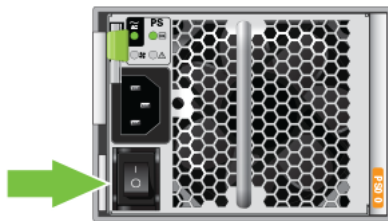
Figure 5.4 Oracle ZFS Storage Appliance ZS5-ES Circuit Breakers
