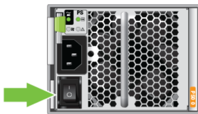
Figure 5.4 Oracle ZFS Storage Appliance ZS7-2 Circuit Breakers
