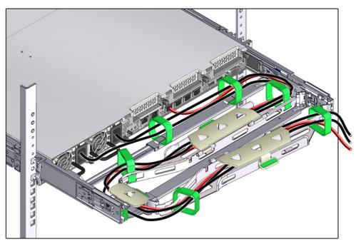
3. Ensure that the secured cables do no extend above the top or below the bottom of the server to which they are attached; otherwise, the cables might snag on other equipment installed in the rack when the server is extended from the rack or returned to the rack.
