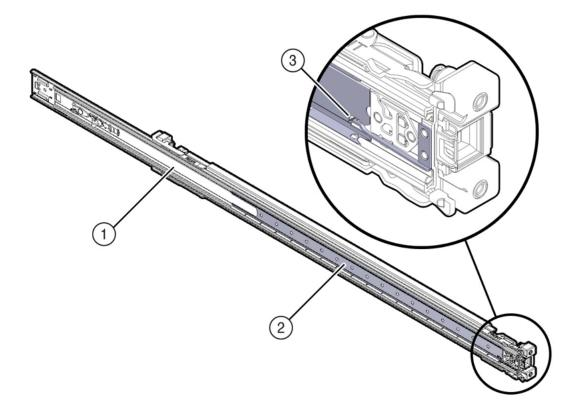
Figure 6.4 Orienting the Slide-Rail With the Ball-Bearing Track
