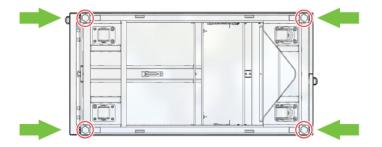
2. Using a 6mm hex wrench, lower the leveling feet to the floor. See Figure 4.4.
