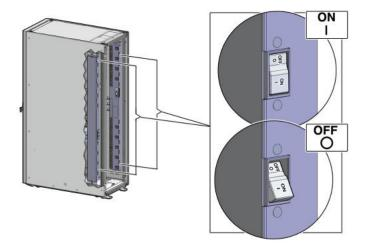
3. Make sure that the circuit breakers located on the rear left and right side power supplies of the Oracle ZFS Storage Appliance ZS7-2 are in the ON (|) position.
