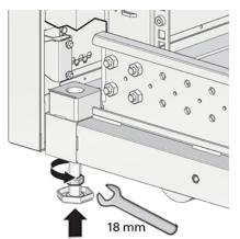
When lowered correctly, the four leveling feet share the load with the casters to increase footprint, improve stability, and help support the full weight of the Oracle Private Cloud Appliance.
