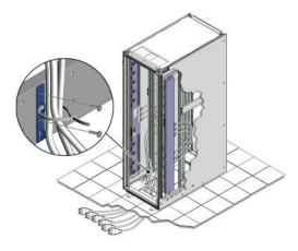
Figure 5.2 Power Cord Routing From the Top of the Rack
