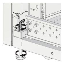
3. Lock the four leveling feet using an 18mm open wrench. See Figure 4.4.
