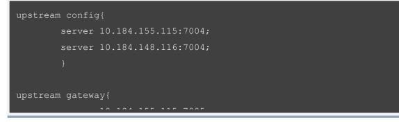
Here there are two load balancers defined. Default load balancing technique: **Round Robin** This block must be placed inside the http block.
