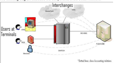
The following diagram illustrates the components in the switch network.
