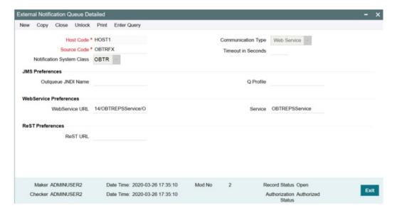
The notification is a call from OBPM to the OBTR Webservice - OBTREPSService that needs to be deployed. The gateway external system setup is required to be done for source code mentioned in the above screenshot. It is important to give the Notification System class as OBTR and communication mode as Web Service.
