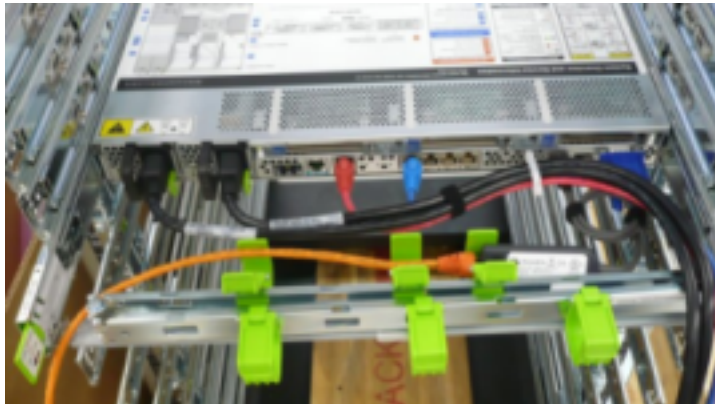
Figure 2-5 Cables Routed Through the Cable Management Arm
