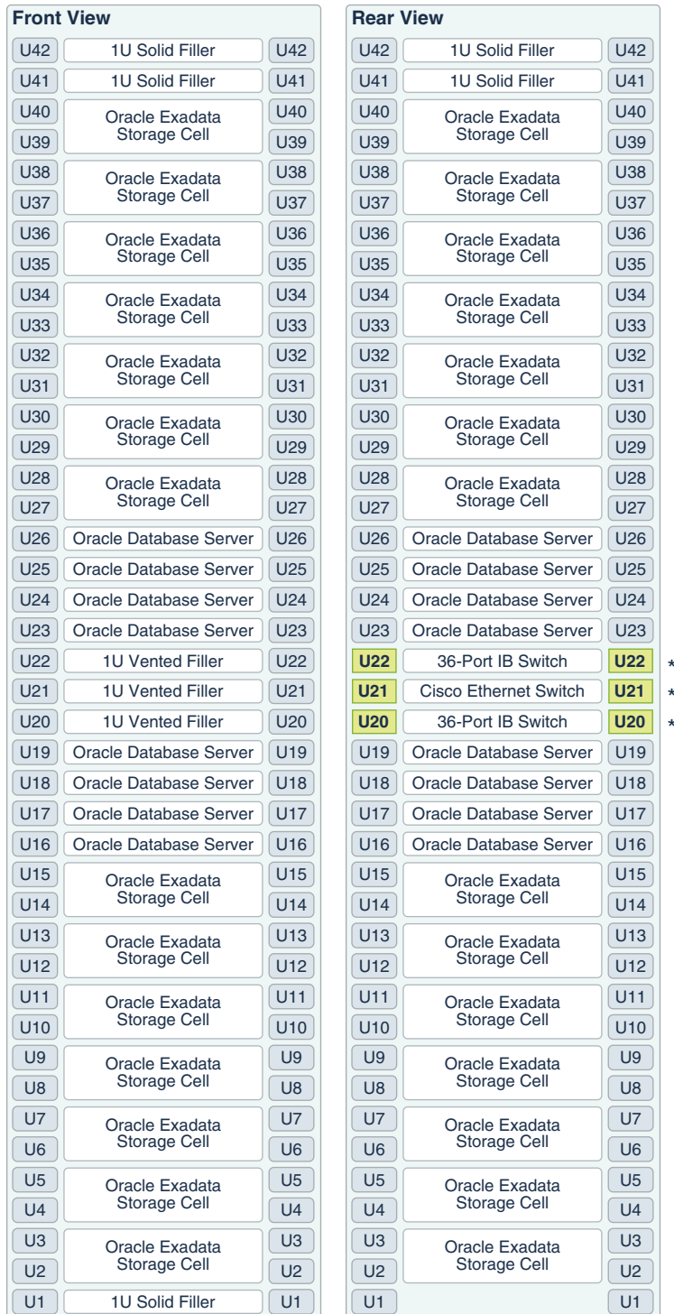
Figure 10-1 Rack Layout of Oracle Exadata Database Machine X8-2 and X7-2 Full Rack
