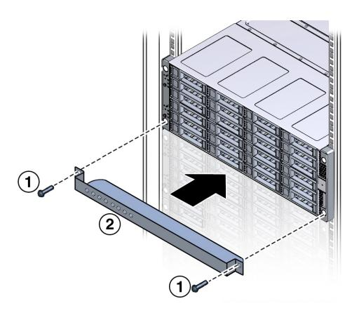
3. Use the two long screws (either the M6 x 30 mm screws or the  $10-32 \times 1.25$  inch screws) [1] to fasten the shipping bracket [2] to the front of the system.
