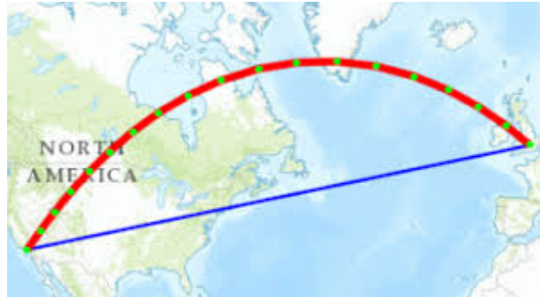
Figure 10-1 Geodetic vs Straight Line
