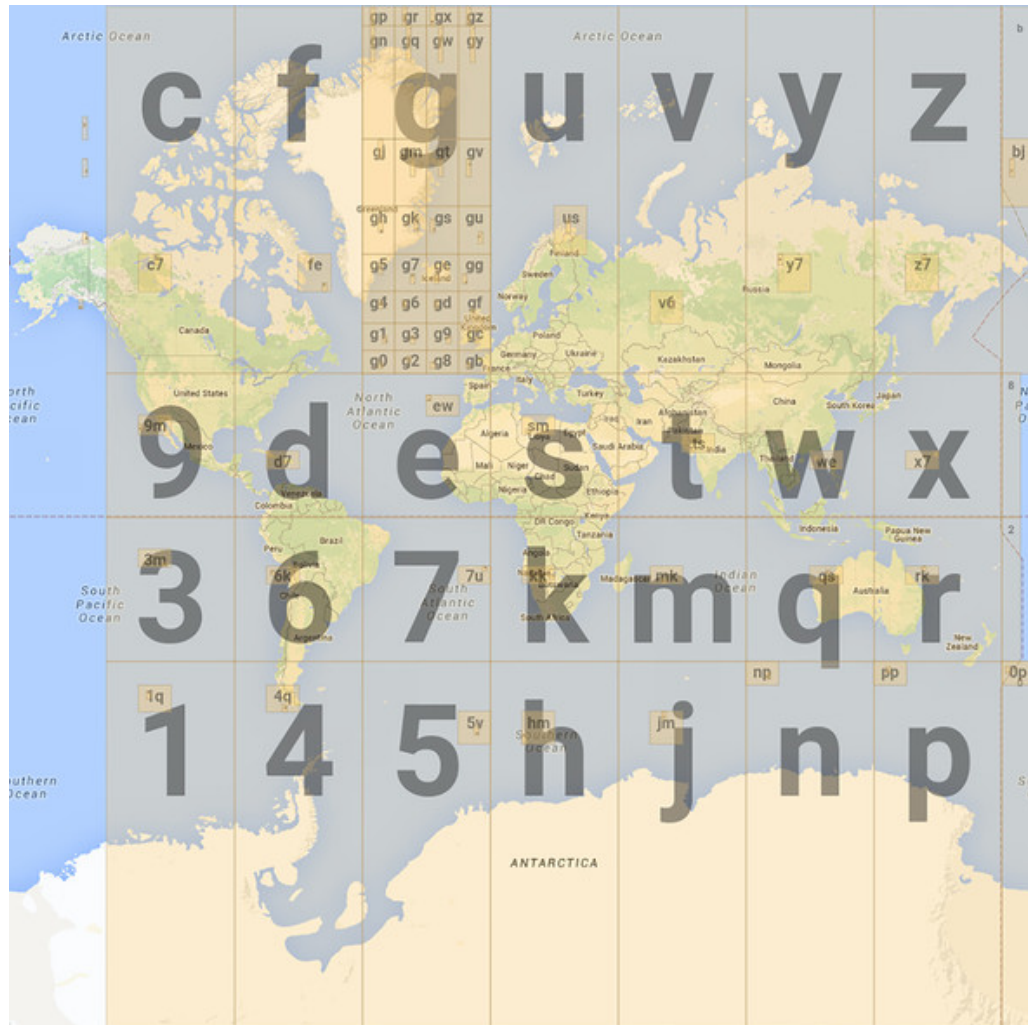
Figure 10-5 Level-1 and Level-2 Geohash Cells
