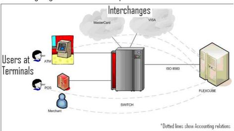
ATMs and POS Terminals are connected with the Switch Software system using proprietary message protocol depending on the upon the terminal device type. Switch software is also connected with 'Interchanges' like VISA and MasterCard.
