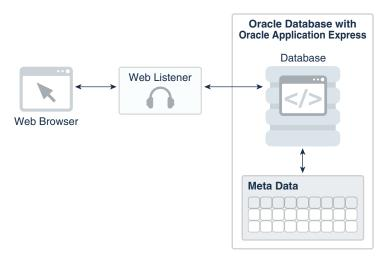
The web listener, Oracle REST Data Services, functions as a communications broker between the Web browser and the Oracle Application Express objects in the Oracle database by mapping browser requests into database stored procedure calls.
