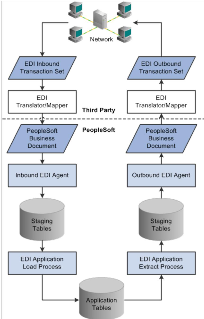
The portion above the dotted line shows the services typically provided by a value-added network (VAN). A VAN provides services related to the exchange of EDI transactions—usually a private network for exchanging EDI transactions, although the network could also be the internet.
