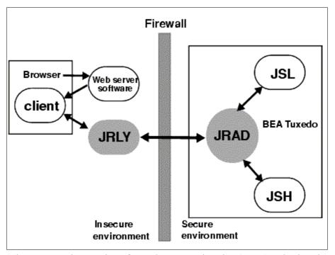
Jolt Internet Relay consists of two elements: Jolt Relay (JRLY) and Jolt Relay Adapter (JRAD). It's important to understand the difference between these two elements.
