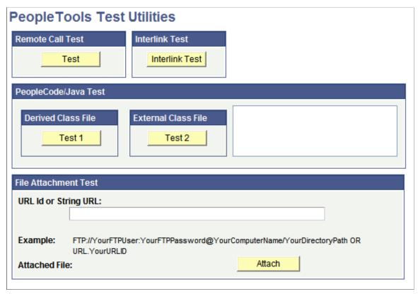
**Remote Call Test** You use the Remote Call Test button to test the Remote Call
