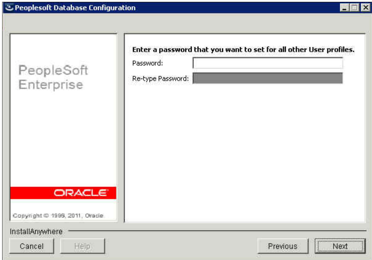
Entering a password for all other User profiles on the PeopleSoft Database Configuration Wizard window
