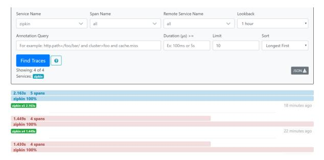
The list of the traces can be seen like the above screen. Some error API calls are made to showcase how to track errors. The blue listings show the successful API hits and the red listings indicate errors. Each block indicates a single trace in the listings.
